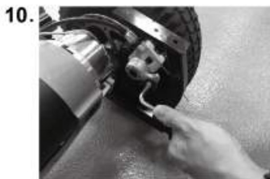
Disconnect the regulating cable. If your scooter without hand brake, please ignore this step.
