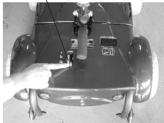
Fig K. Move release bar backward to free wheel mode. (Right motor)
